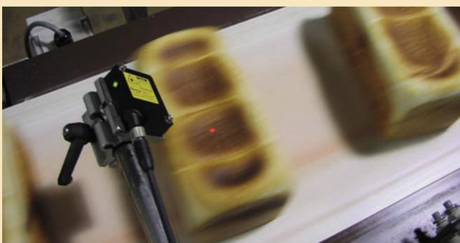
Laser technology developed by Crop & Food Research's Arran Wilson to measure collapse of loaves.
